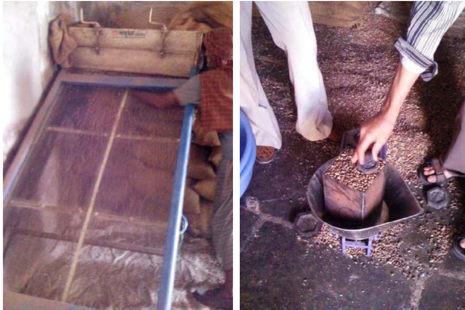
Figure 3.3: The sieve (left) and the 4.2litre container (right) used to check the foreign matter content and weight (Image source: Sinha, 2009)
