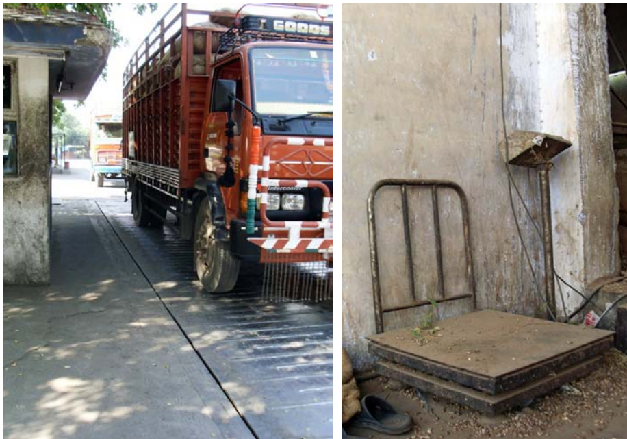
Figure 3.2: The electronic weigh bridge (left) and the electronic scale (right) used for weighing the commodities at that hub.
