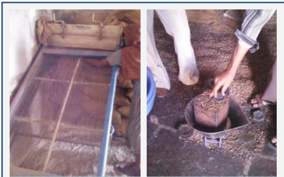
**The sieve (left) and the 4.2litre container (right) used to check the foreign matter content and weight**
