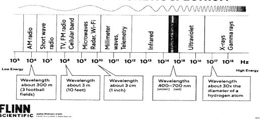
Radio waves in the above diagram include TV, FM radio, Cellular band, short wave and AM radio waves. As can be observed, they have a low frequency and long wavelength, and are significant from a standpoint of human utility. This is because all telecommunication (whether it be broadcasting television programmes or long-distance telephone calls or accessing the internet via Wi-Fi) happens through radio waves.
